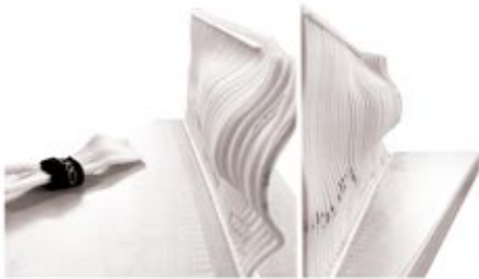
Phase 1 Facade panels 3D printed and grouped into sub-groups of two. One Facade after glued and painted, ready to be joined with the other parts into one final model.
